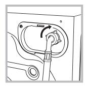
2. Connect the inlet hose to the washerdryer by screwing it onto the corresponding water inlet of the appliance, which is situated on the top right-hand side of the rear part of the appliance (see figure).
